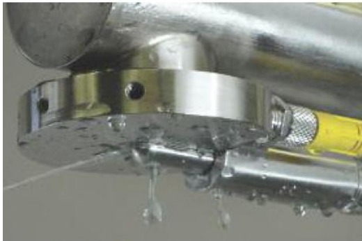
Dosing valve shut
